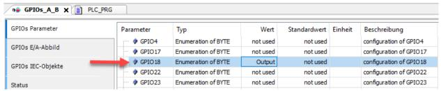
Figure 27: CODESYS - GPIO18 as an output
