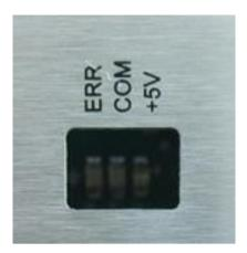
Figure 4: Status LEDs "ERR", "COM" and "+5V" on PiXtend elO devices
