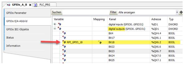
Figure 28: CODESYS - GPIO18 as a variable
