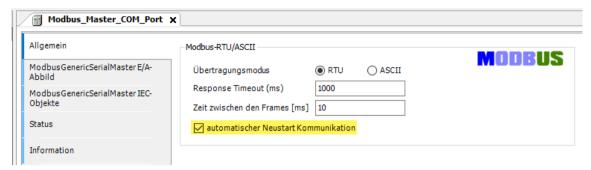
Figure 41: CODESYS - Modbus Master settings
