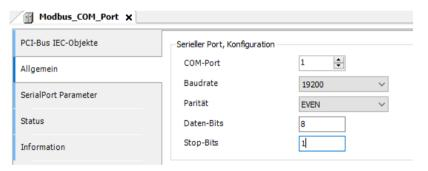
Figure 20: CODESYS - serial settings
