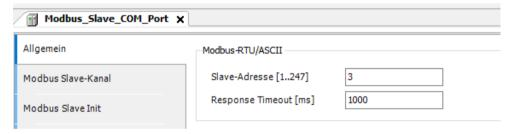
Figure 42: CODESYS - Modbus Slave settings
