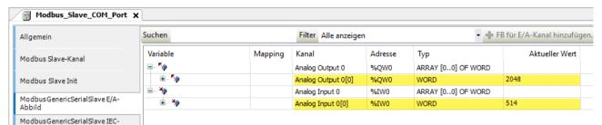
Figure 51: CODESYS - Modbus slave analog output 0 and analog input 0
