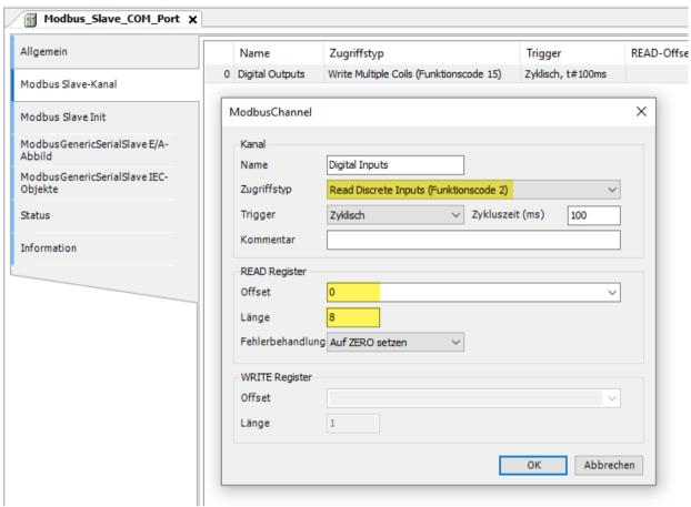
Figure 24: CODESYS - Create Modbus Slave communication channel (2)
