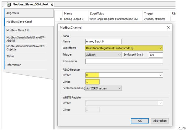
44: CODESYS - Create Modbus communication channel (2)
