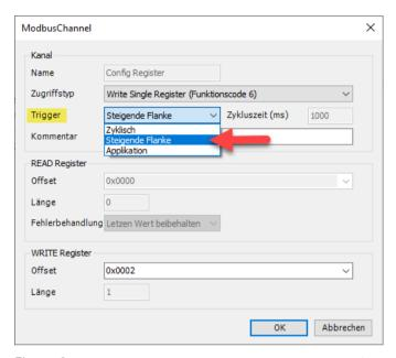
Figure 3: CODESYS Modbus, Transfer via trigger variable (rising edge)
