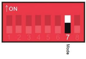
Figure 9: DIP block 2 - CONFIG - mode - PiXtend elO Protocol
