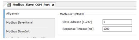
Figure 22: CODESYS - Modbus Slave settings
