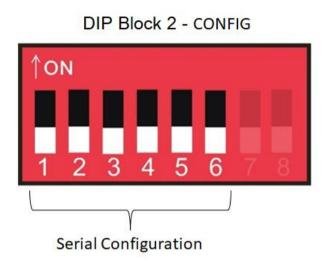
Figure 7: DIP block 2 - CONFIG - serial configuration
