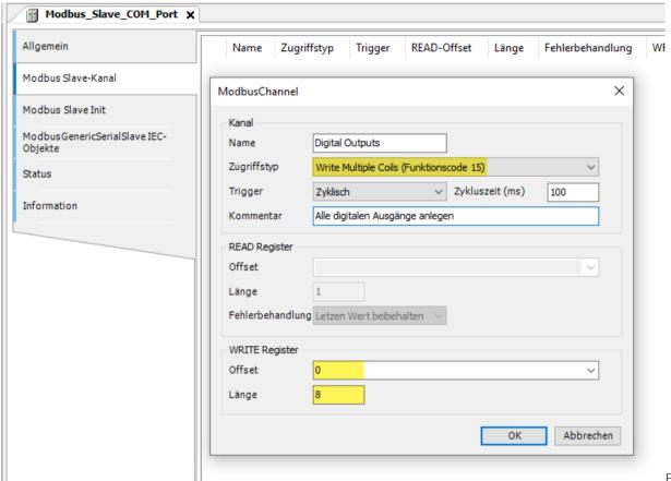
23: CODESYS - Create Modbus Slave communication channel
