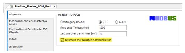
Figure 21: CODESYS - Modbus Master settings
