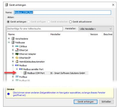
Figure 17: CODESYS - Add device window
