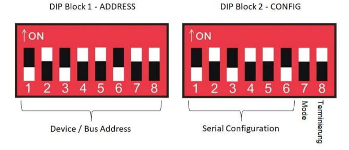
Figure 5: Device configuration - overview DIP switches - scheme  $\,$
