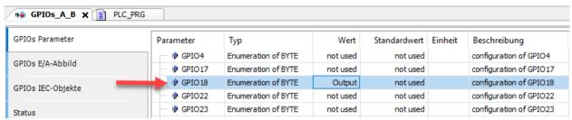
Figure 47: CODESYS - GPIO18 defined as an output
