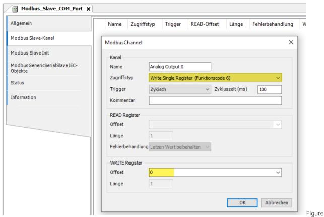
43: CODESYS - Create Modbus communication channel (1)
