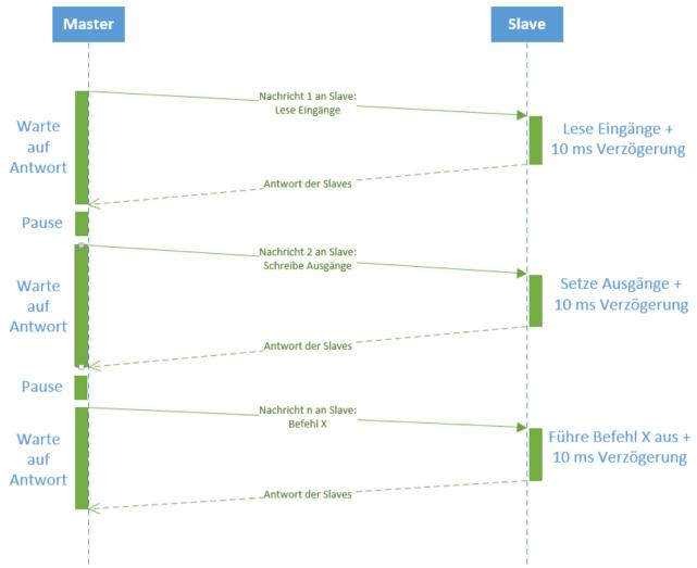
Figure 54: PiXtend eIO protocol - Communication - process overview
