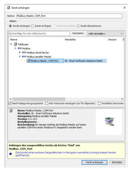
Figure 18: CODESYS - Add device - Modbus master
