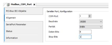
Figure 40: CODESYS - Modbus serial settings
