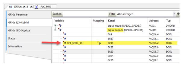
Figure 48: CODESYS - GPIO18 as a variable
