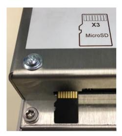
The microSD card must be inserted with contacts to the rear (towards the rear of the device) as shown in the figure above.
