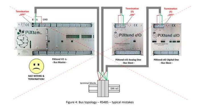
There are different network topologies. However, star, tree, ring and mesh networks are not suitable for RS485 and therefore also not for PiXtend eIO connections. RS485 is always set up as a line or in a bus structure.
