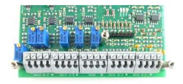
Figure 40: Terminal blocks - analog inputs and outputs
