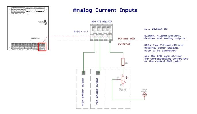
Figure 44: Simplified wiring diagram: connection of the analog current inputs
