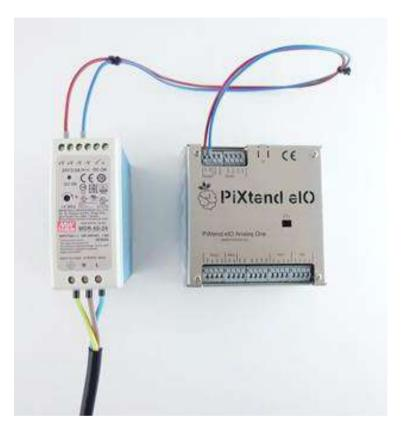
Figure 27: 24V; 2.5A DIN rail power supply connected to the PiXtend eIO
