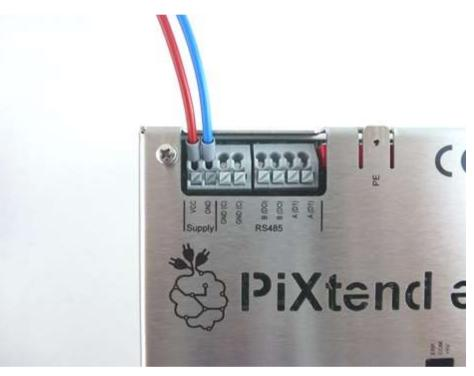
Figure 25: Power connection to the PiXtend eIO
