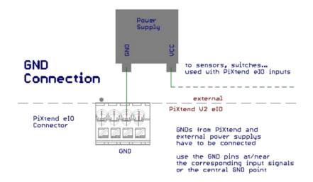
Figure 37: Simplified wiring diagram: GND connection
