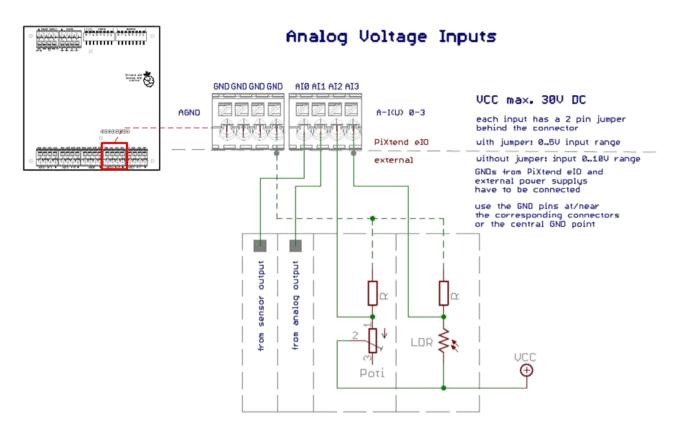
Figure 42: Simplified wiring diagram: connection of the analog voltage inputs
