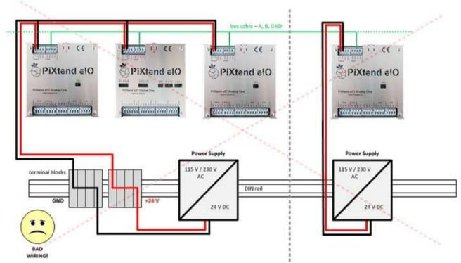
Figure 2: Topology of the power supply – typical mistakes
