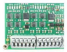
Figure 38: Terminal block - digital outputs
