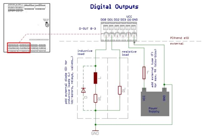
Figure 39: Simplified wiring diagram: connection of the digital outputs
