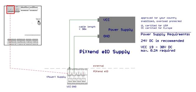
Figure 31: Simplified wiring diagram: connection of the central power supply
