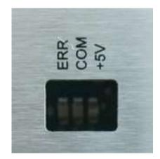
Figure 32: Status LEDs "ERR", "COM" and "+5V" on PiXtend eIO modules
