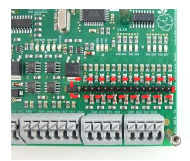
Figure 19: Jumper - digital inputs in 24V range (factory default)
