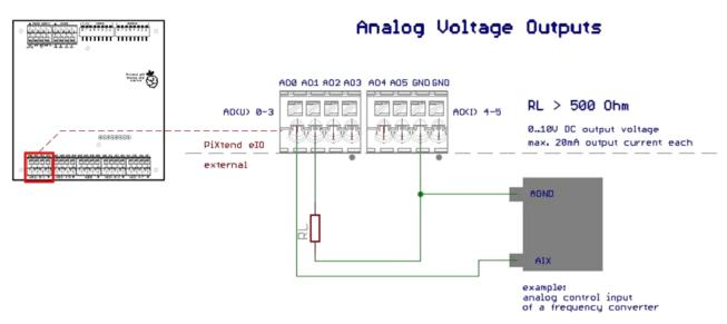
Figure 46: Simplified wiring diagram: connection of the analog voltage outputs
