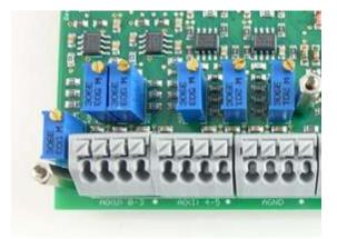
Figure 45: Terminal block – analog outputs
