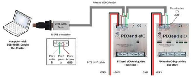
Figure 29: Test setup - PC with USB RS485 dongle as master
