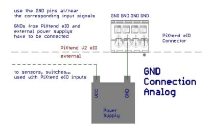
Figure 43: Simplified wiring diagram: GND connection
