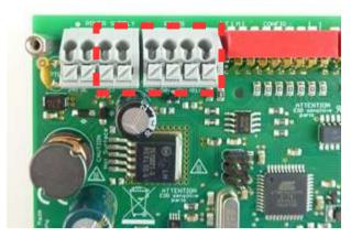
Figure 33: Terminal block connector - RS485 interface
