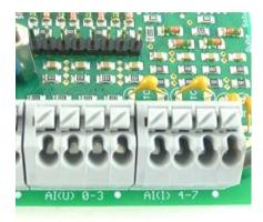
Figure 41: Terminal block - analog inputs
