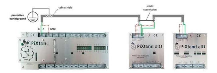
Figure 5: Shielded bus cables - shield connection
