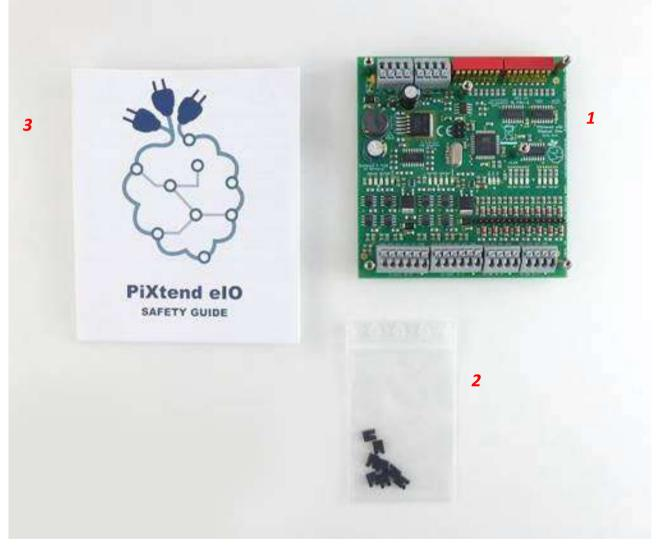
Figure 6: Package contents: PiXtend eIO Digital One Basic (Article 50199 007)
