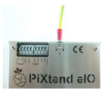
Figure 21: Grounding connection (PE) on the PiXtend eIO cover
