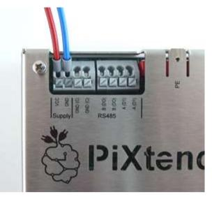
Figure 30: Terminal block for the power supply
