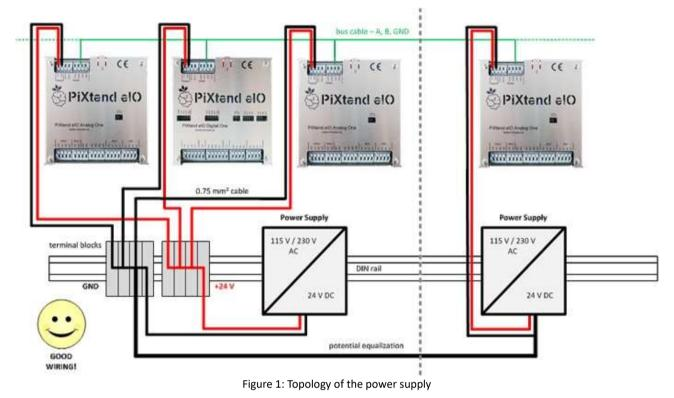
Figure 1 shows the correct wiring, power supply topology for several PiXtend eIO devices. Each device is connected separately to a common supply or ground point with its own lines.
