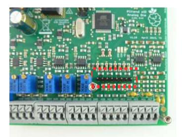
Figure 20: Jumper - analog voltage inputs in 10V range (factory default)
