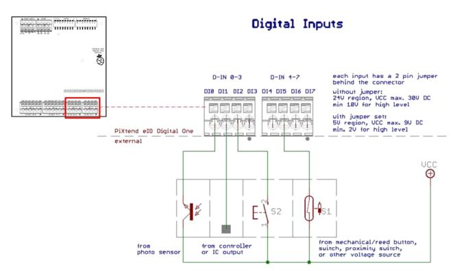
Figure 36: Simplified wiring diagram: connection of the digital inputs
