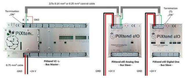
Figure 28: Test setup - PiXtend V2 -L- as master
